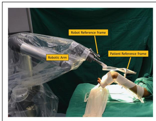
**Figure 1.** The wrist is extended and securely affixed to a wrist positioning jig. The patient reference frame is fixed onto the positioning jig. The robot reference frame is attached to the robotic arm.
