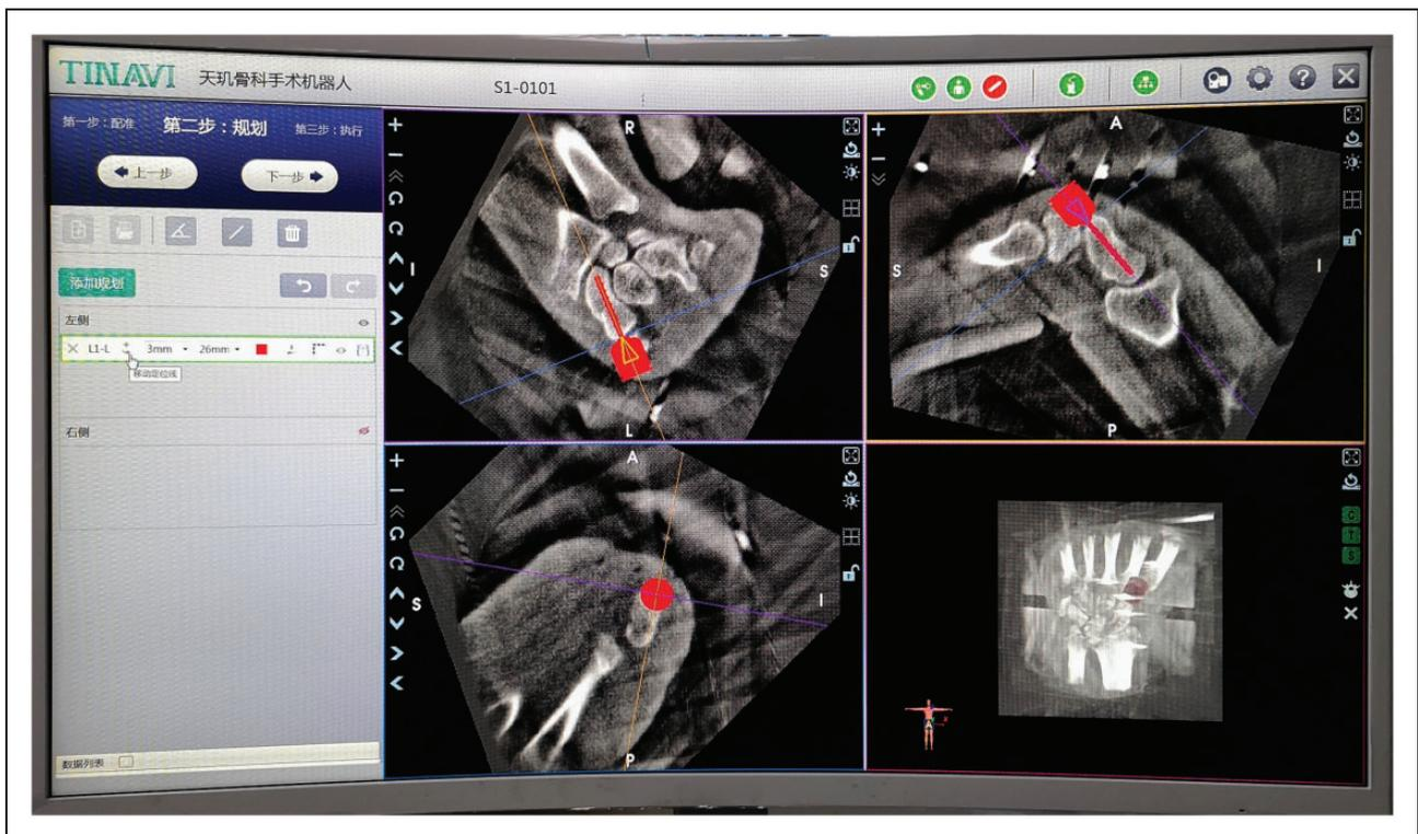
**Figure 3.** Graphical user interface of the surgical planning software in the TiRobot workstation. The surgeon can determine the optimal screw trajectory in the central zone of the scaphoid by modifying the screw path in the sagittal, axial and coronal planes.
